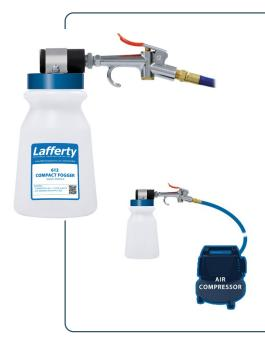
The 612 Compact Fogger is a damp mist sprayer that uses compressed air (1.2 CFM @ 80 PSI) and venturi action to draw ready-to-use chemical solution from the attached bottle and project it up to 6 feet. The adjustable output can wet surfaces at close range or spray mist (fog) into the air to cover exposed surfaces and penetrate hard-to-reach areas. The low CFM requirement of this unique fogger allows it to be used with smaller consumer-grade air compressors.
